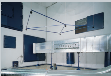
Reverberation chamber for acoustic measurements
