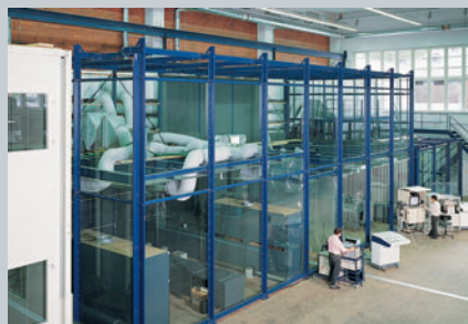
One of the room airflow test rooms
