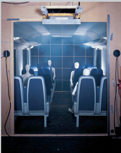
Airflow test, 1:1 scale, to confirm passengers' thermal comfort.
